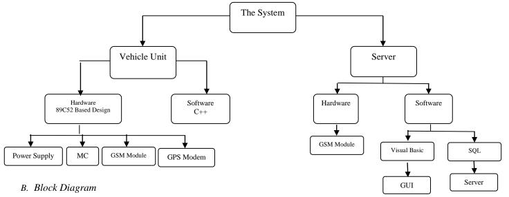
The Block Diagram of the system is given below.
