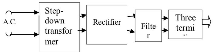
Fig.6 Block Diagram of Power Supply
