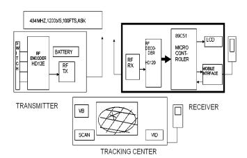
Tracking centre sends the VID(vehicle ID) as an SMS to the cell phone that is connected with the receiver being fixed in the corresponding vehicle which is currently present in a particular cell.
